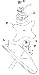
Hook the blade guard/combination guard (A) onto the fitting on the shaft and secure with the bolt. **CAUTION!** Use the recommended blade guard. See the Technical data section.
